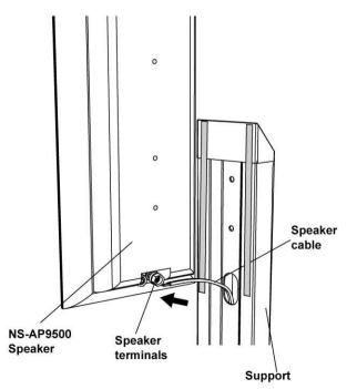
7 Fix the speaker cable to the base with the cable protection seal.
