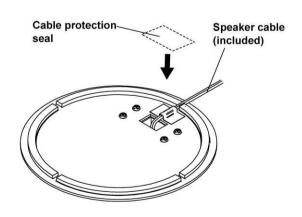
Assembly is complete Assemble the other stand in the same way.
