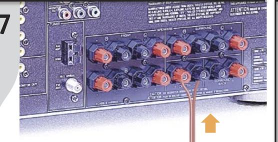
Connect Center Speaker Positive (+) side of the wire with white stripe attaches to (+) terminal. Negative (-) side attaches to (-) terminal. **CAUTION** Receiver must not be plugged in while connecting speakers.
