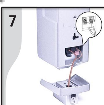
Connect Front and Surround Speaker Wire Positive (+) side of the wire with white stripe attaches to (+) terminal. Negative (-) side attaches to (-) terminal.
