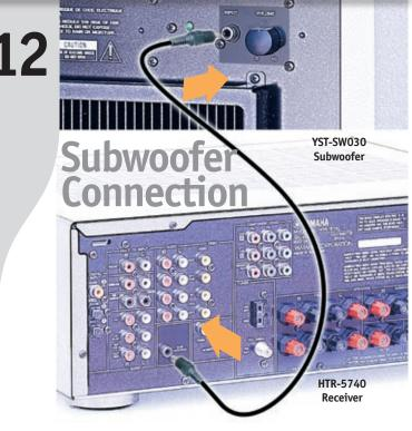
Connect RCA Cable Connect RCA cable 8 to subwoofer 4. Set subwoofer VOLUME control to half-way mark and POWER to OFF. Connect RCA cable to receiver from subwoofer.
