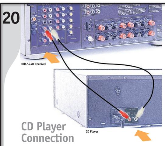
Connect CD Player (optional) Connect RCA audio cables (not included) to "CD" terminals on receiver as shown. If your CD Player has digital output terminal, connect digital cable (not included) to HTR-5740 Receiver Digital Input terminal. See page 17 of your HTR-5740 Owner's Manual for more information.
