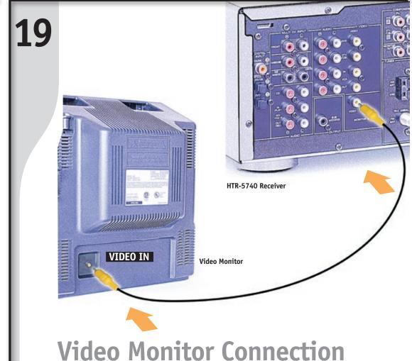
Connect a Video Monitor (optional) Connect an RCA video cable (not included) to receiver Monitor OUT from your video monitor as shown.
