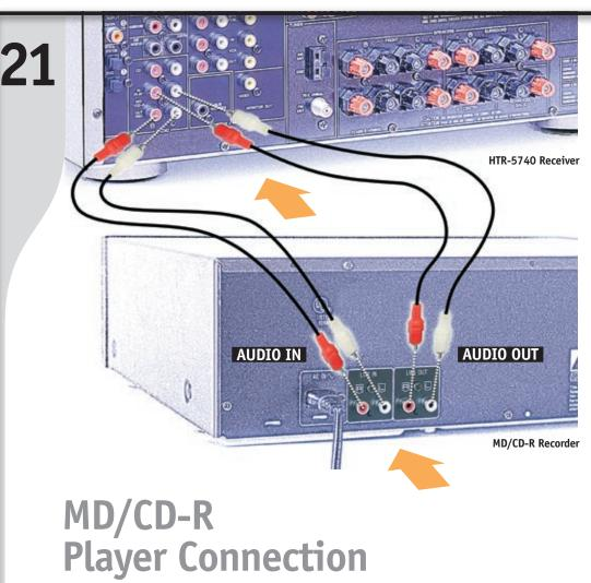
Connect MD/CD-R Recorder (optional) Connect RCA audio cables (not included) to "MD/CD-R" terminals on receiver as shown.
