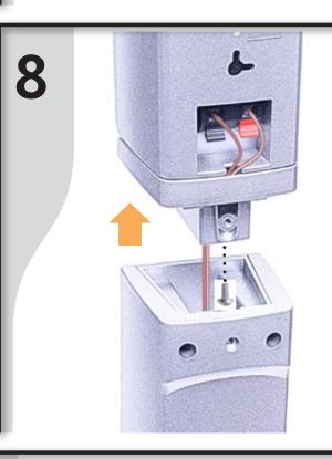
Attach Adapter to the Speaker using the supplied screw
