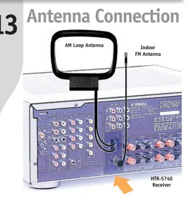
Connect Antennas to Receiver Locate AM loop antenna and indoor FM antenna. Keeping receiver unplugged, connect as shown. For more information about obtaining clear reception and grounding, see your Owner's Manual.
