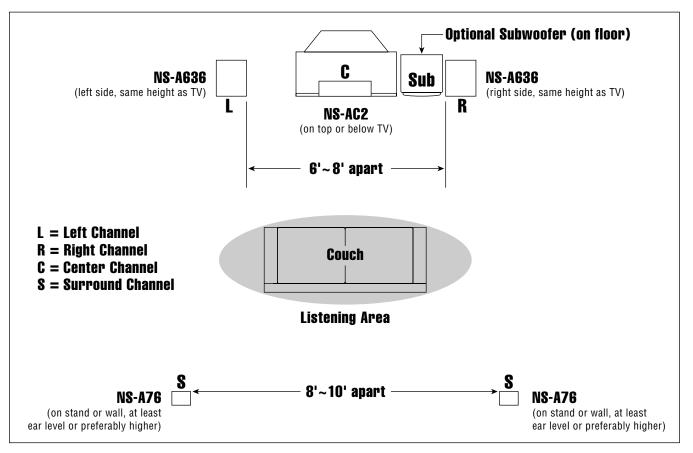
*Figure 1. This overhead view shows a typical system layout for the YHT-10 Home Theater speaker package.*
